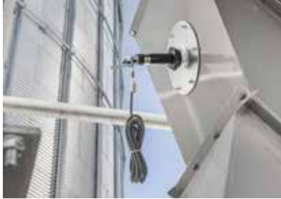
Plug switch option in head discharge eliminates potential overload concerns.
