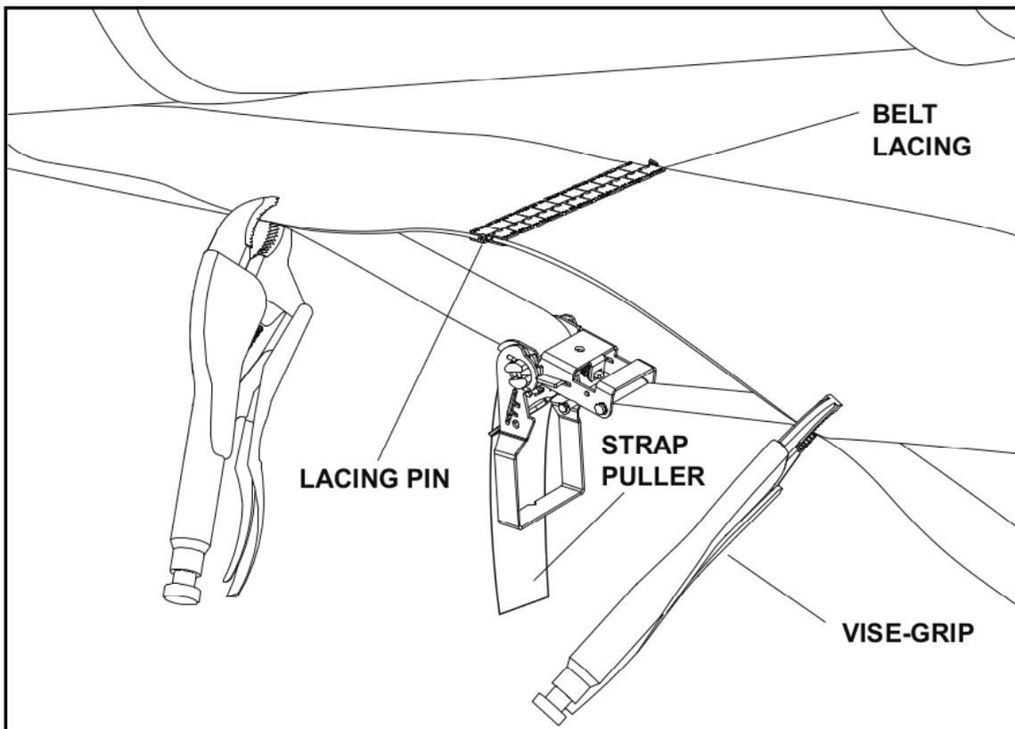
9. Install the lacing pin and crimp the retainer clips onto each end of the lacing pin, see [Figure 18.](#)
