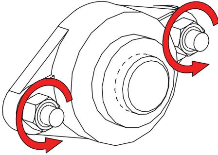
2. Rotate adjustment bolt 1/2 turn.
