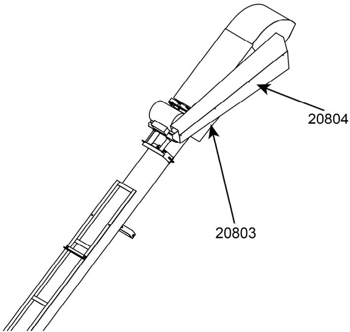
**Figure 5. Hydraulic Drive Safety Decal Location**
