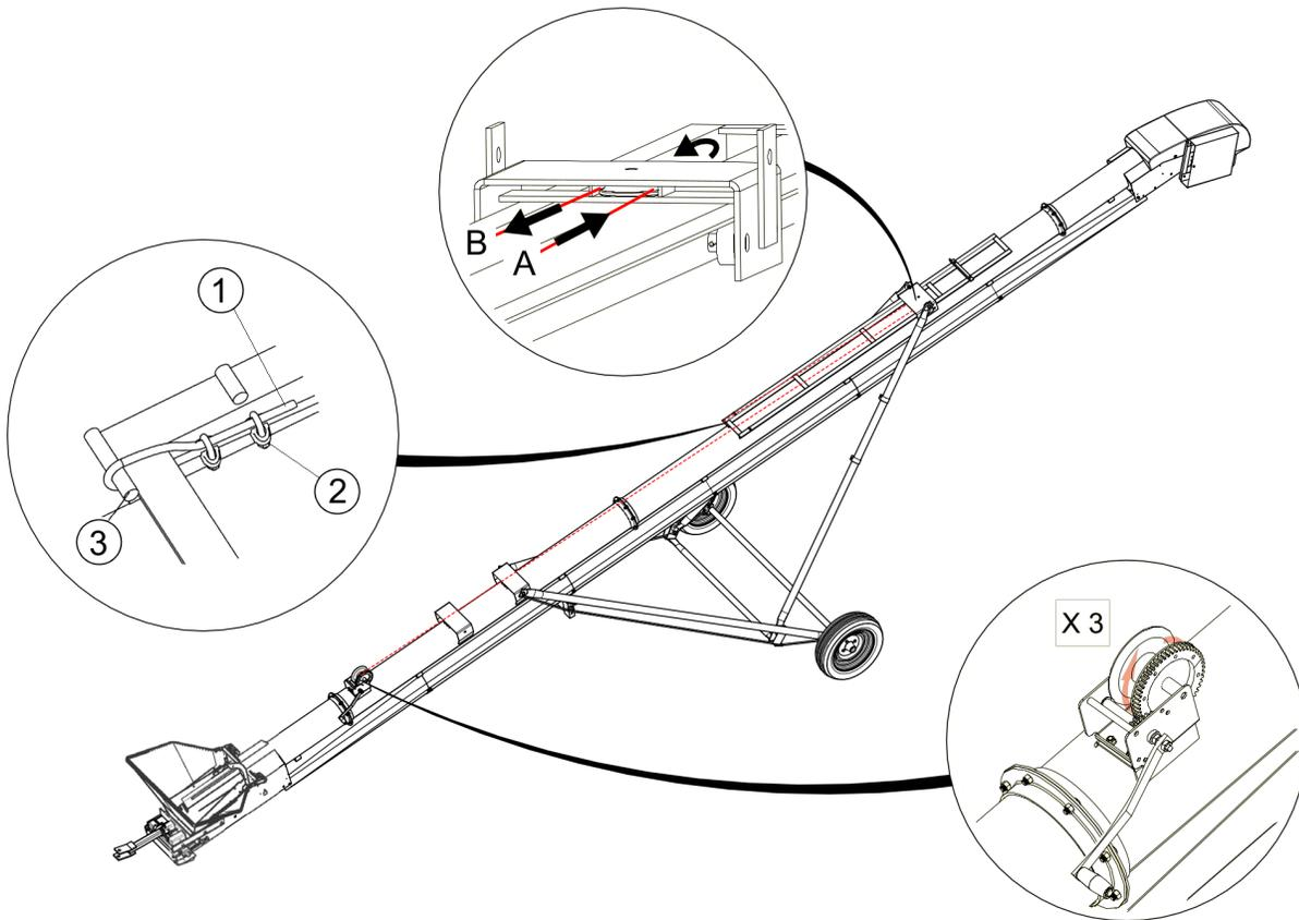
**Figure 33. Winch Drum and Lift Cable**
