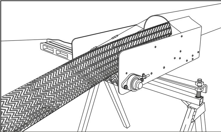
2. Wrap the belt around the spout roller and pull it back under the conveyor tube to the hopper until approximately 6' (1.8 m) of excess belt remains on the stand behind the hopper.
