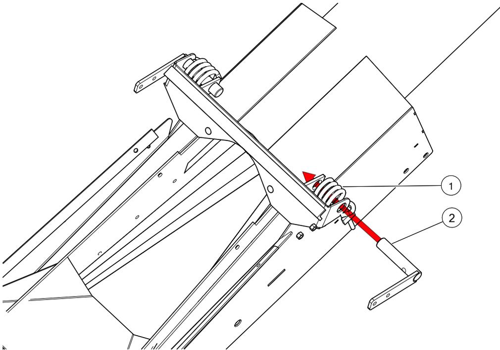
3. Clip the hopper springs over the tabs on the hopper and shaft bracket (see [Figure 24](#)).
