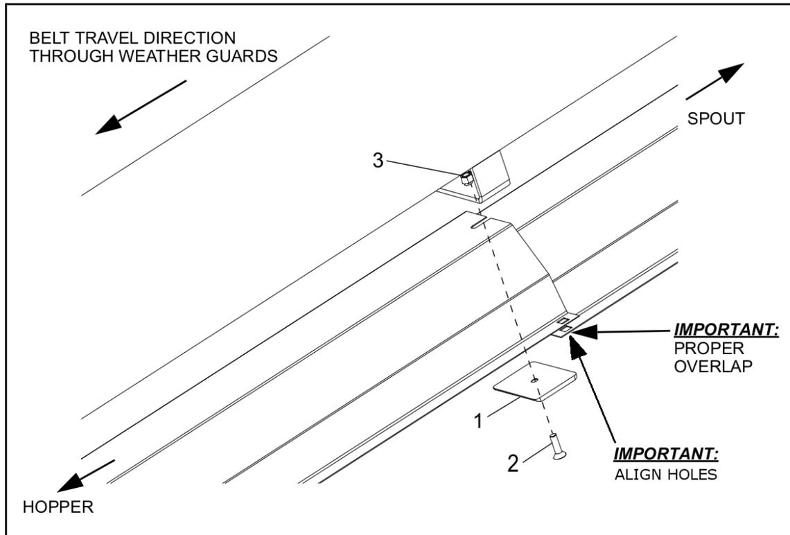
**Figure 11. Weather Guard Section Locations (WCX 1335)**
