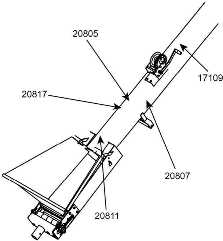
**Figure 2. Electric Top Drive Safety Decal Locations**
