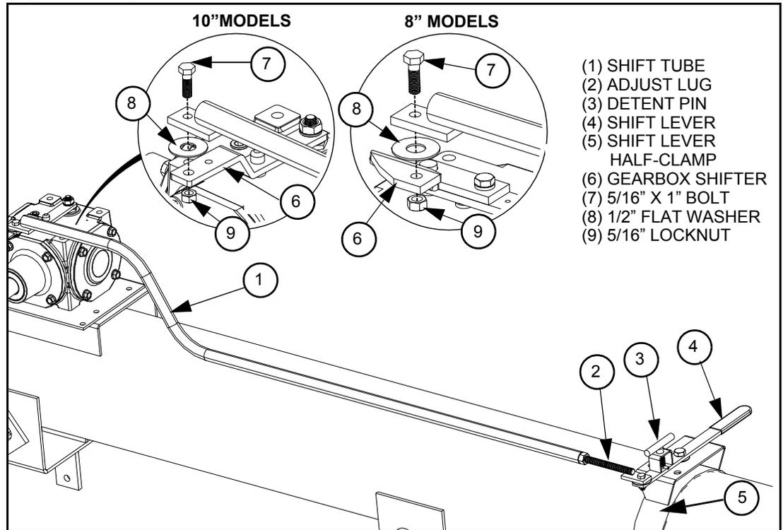
**Figure 2 Shift Lever and Lower Shift Tube Attachment**
