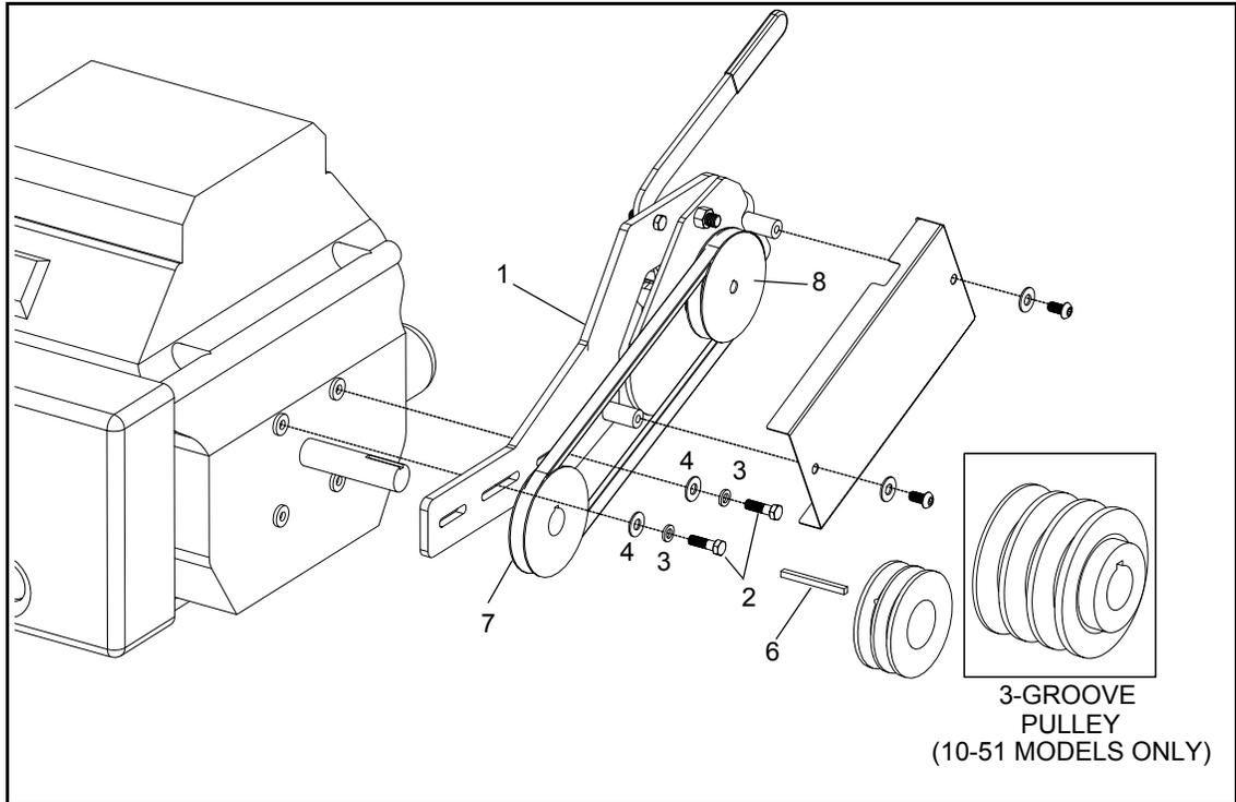
**Figure 3.2 Hydraulic Pump Bracket Installation (Vanguard Engine)**
