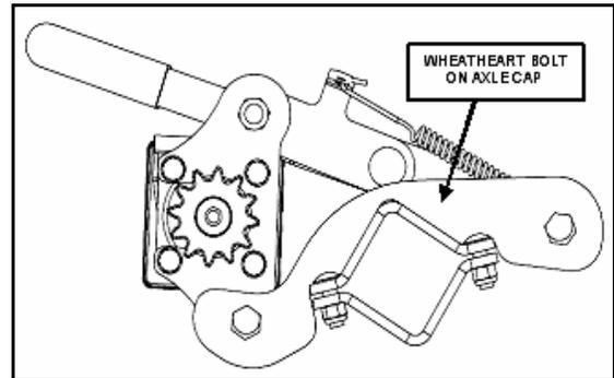
3. With the pinion gear flush with the ring gear (Figure 3.6), bolt the axle cap to the axle tube with four carriage bolts and lock-nuts.
