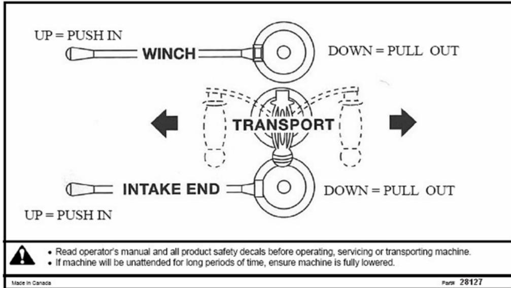
**Figure 5.2 Hydraulic Control Valve**
