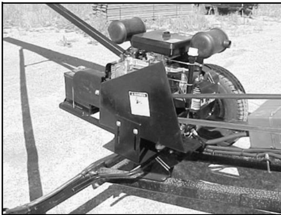
**Figure 3.3 Belt Engaging Lever & Engine**
