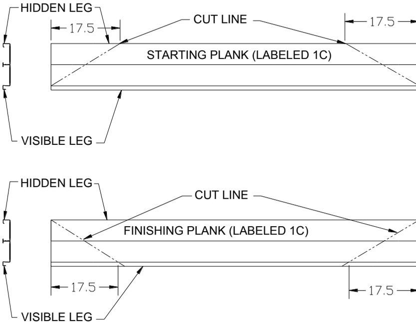
**All other planks:** All of the other planks that are required to be cut (2C, 3C and all others labeled with a C) are cut at 45° angle (as illustrated). In this case the ends of the cut are 10” from the ends of the plank. Again planks on opposite sides of the bin are cut differently as per the Important Note above. Sometimes on larger bins a split plank is also a cut plank. In these occasions only one end of each split plank pair is cut.
