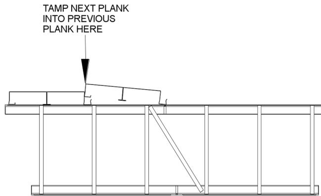
4. Using the preceding instructions, and the appropriate floor plank and support drawings, install the remaining floor supports and planks:
