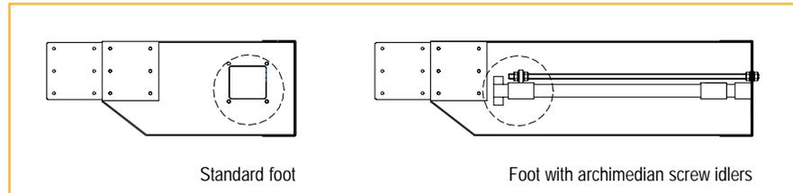
The machine has been designed in two versions - with and without Archimedean screw idlers. In the first case, the tensioning of the belt is done by means of a pair of Archimedean screw idlers which act on the return drum unit. Generally, this system is suitable for machines of limited length (side card) since the specifications of the large belts used and the functioning principle of these machines entail different manufacturing solutions to recover the belt's natural stretching and elasticity.
