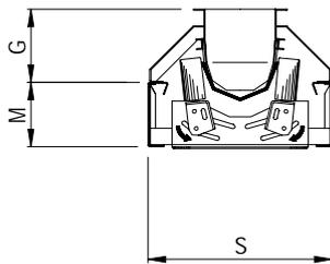
Discharge tripper section
