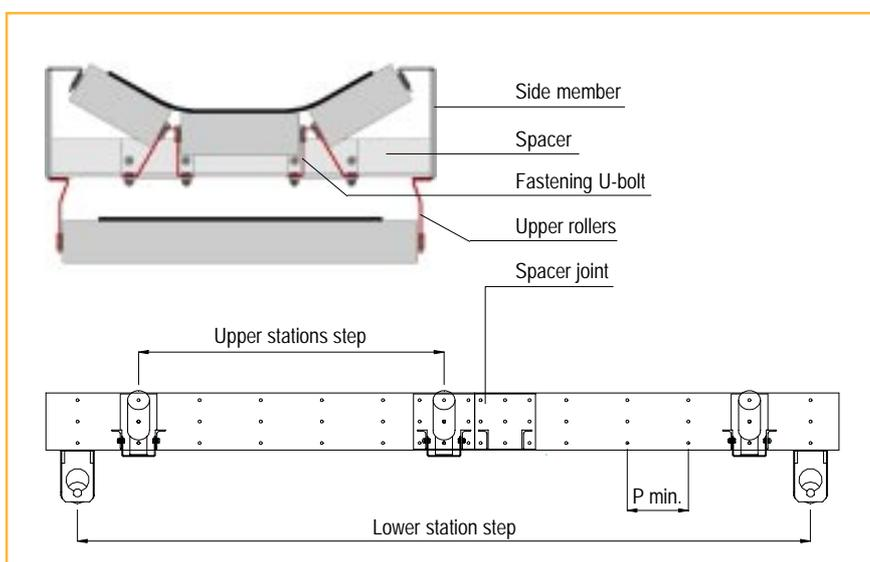
The following card records the main manufacturing specifications of the upright supports for the various series of conveyors. The feed rollers, due to a special profile of the side
